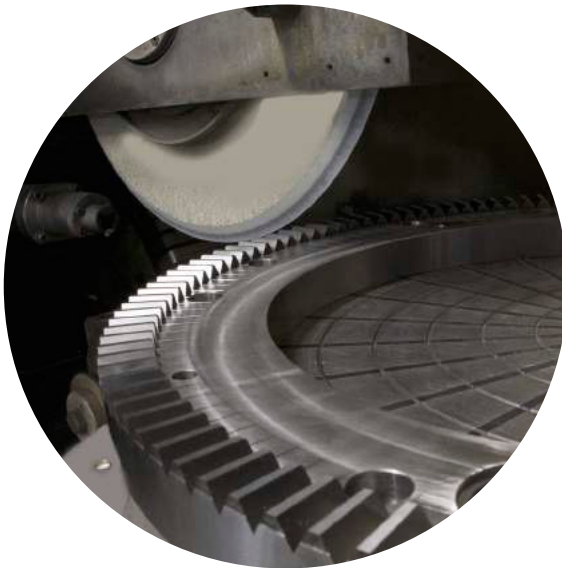
~ Rettifica denti ~ Teeth grinding
